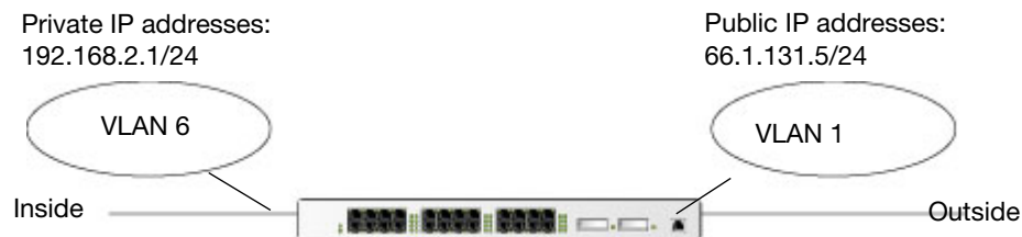
Figure 5 Example: Source NAT using Switch IP Address
